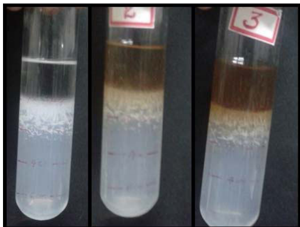
Figure 3: The invitro growth of struvite crystals in test tubes
