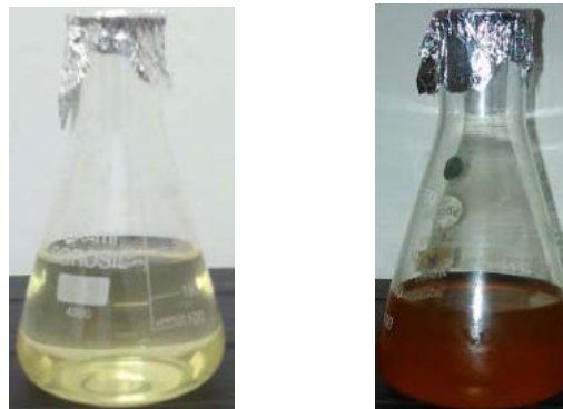
Figure 6: Colour change in reaction mixture (Silver nitrate + Myrica nagi leaves extract) (a) at 0 hours; (b) after 2hours
